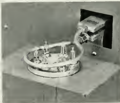
ELECTRONIC METHOD OF SOLDERING TERMINALS ON TRANSFORMER CANS.
